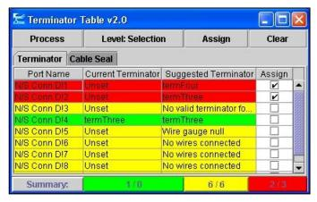
TermTable quickly highlights errors and allows you to correct them easily
